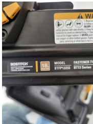
Bostitch BTFP12233: the actual label shows the model and 18-ga size.
